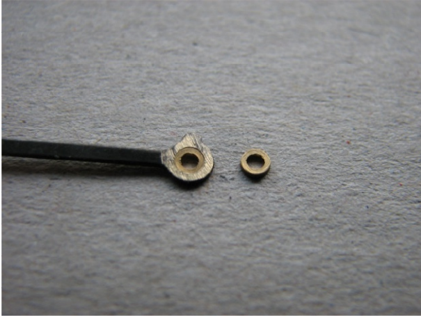
Bush in rod ready for soldering.
