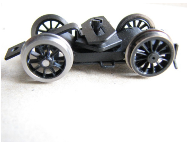
One Gibson wheel set installed
