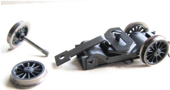
One Hornby wheel removed
