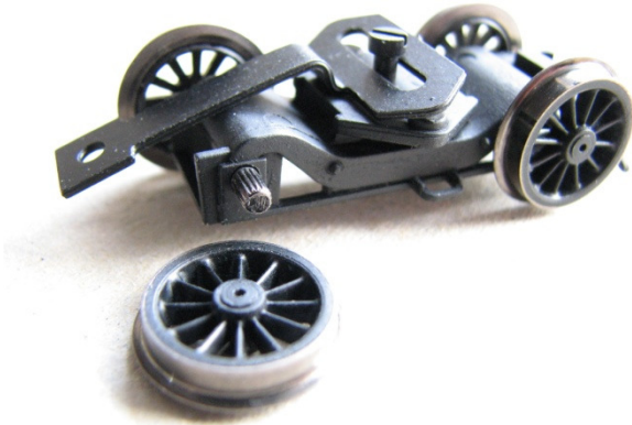
One Hornby wheel removed
