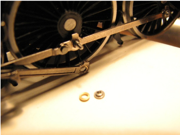
Bush to space Connecting rod from coupling rod.
